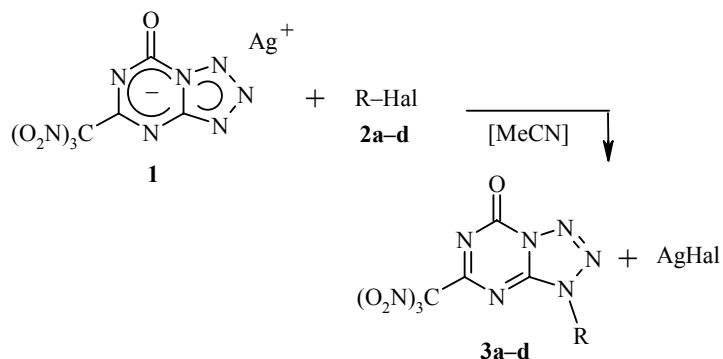
**2 a** R = *i*-Pr, Hal = I; **b** R = (CH<sub>2</sub>)<sub>4</sub>Me, Hal = I; **c** R = Bn, Hal = Cl; **d** R = CH<sub>2</sub>COAd, Hal = Br;
